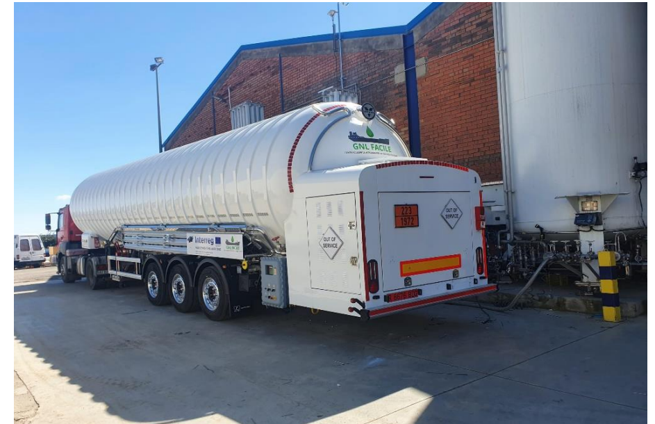
55 m 3 de GNL Fully Automatic
