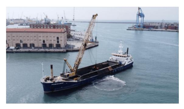
Dredging operations are underway across the Ports of Genoa and Savona, with the dual objective to maintain and to deepen the depth alongside quaylines to cater for the arrival of the next generation ultra- large vessels, both full-container and cruise ships. It is essential to remove regularly from the navigation channels the accumulations of sand and sediment deposited by tide and river flows into the sea to ensure safe and easy access to terminal facilities.
