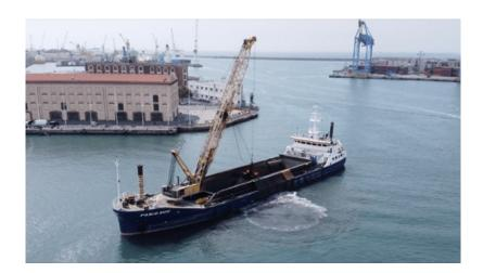
Dredging operations are underway across the Ports of Genoa and Savona, with the dual objective to maintain and to deepen the depth alongside quaylines to cater for the arrival of the next generation ultra- large vessels, both full-container and cruise ships. It is essential to remove regularly from the navigation channels the accumulations of sand and sediment deposited by tide and river flows into the sea to ensure safe and easy access to terminal facilities.
