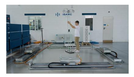
The 65-metre high glass and steel control tower, under construction in Genoa's Levante Waterfront, will be equipped with a technologically innovative system designed to protect the building from vibrations caused by strong winds and severe sea conditions. Tuned mass dampers will be programmed and activated by electrical engines, across the Electro Pro system planned and built by ISAAC, to counteract all possible swaying motions of the tower and eliminate vibrations.
